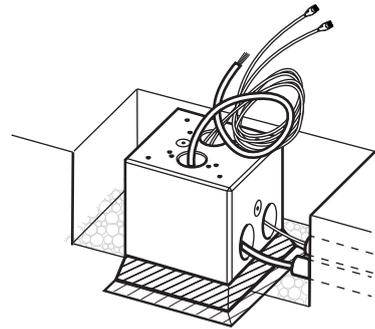
7 Run data cables with sufficient length (approx. 2.0 m) through the same or the second empty conduit for the subsequent installation of the wallbox on the mounting pole.
