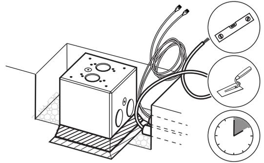
5 Allow the concrete to set completely over a reasonable period of time so that the foundation is protected from slipping when the ditch is eventually filled and compacted with compactable soil.
