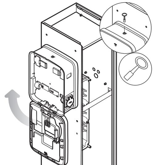
**12** Using the slotted screwdriver and a hammer, knock out one of the pre-stamped M20 cable entries on the top of the small distribution board.
