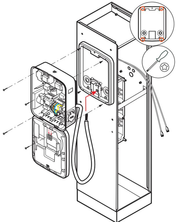
**8** Run the data cables through the small cable outlets of the mounting pole and into the housing of the wallbox.
