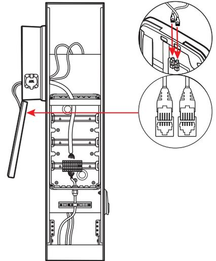
**9** Connect the data cables to the Modbus interfaces on the inside of the wallbox housing cover.
