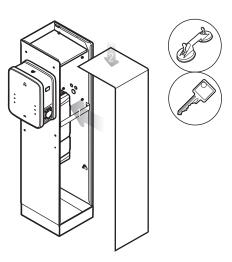
**8** Lock the housing cover of the POLEMH6 with the double cylinder pivot lever.
