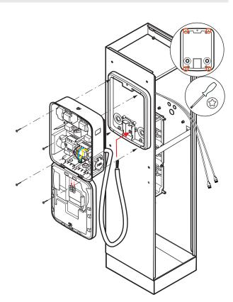
7 Screw the wallbox into the mounting plate using the Torx screwdriver and the screws supplied with the wallbox.
