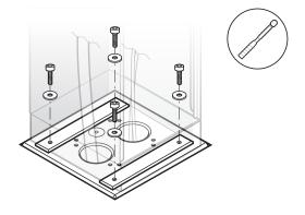
**5** Use the slotted screwdriver to loosen the eight screws in the upper part of the small distribution board and pull off the upper part.
