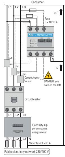
Figure: Connection for indirect measurement with current transformers
