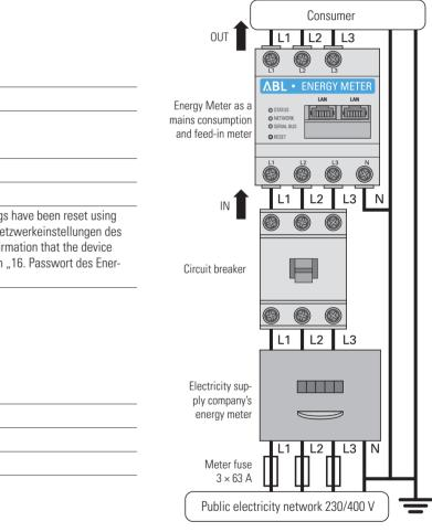
Figure: Connection for direct measurement
