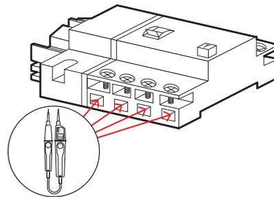
3 Use the installation tester and the vehicle simulation adapter to conduct all other required checks.
