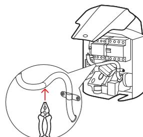
2 Insert the individual conductors of the power supply cable into the respective terminals of the RCCB and tighten them using the Phillips-head screwdriver.
