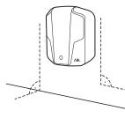
■ The mounting surface must measure at least 273 x 222 mm (height x width). Overhangs caused by the charging socket or the stored charging cable are not included in these dimensions.
