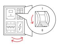
The Wallbox eMH1 is no longer connected to the electricity grid and can be removed by a qualified specialist electrical contractor if required.
