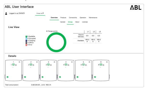
The **Live View** shows all eM4 chargers within the charging group with their current status and the consumption of all connected electric vehicles per phase.
