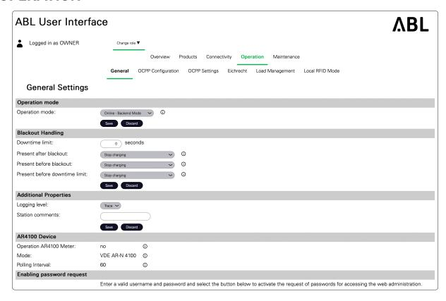
The **Operation** tab shows details about the various communication interfaces and protocols within your current installation.
