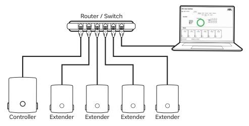
In this scenario, the computer is connected with an eM4 charging group via an external router or switch.
