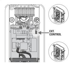
After establishing the electrical connection of the control cable, the remote disconnection function must be activated via the ABL **Configuration App**. To do this, please refer to the sections starting on page 40.
