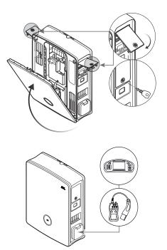
→ Use an installation tester and a vehicle simulation adapter to conduct the prescribed tests.
