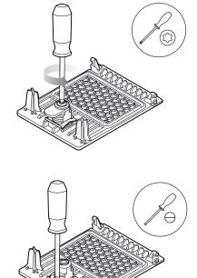
${\bf 5} \ \ {\rm Remove \ the \ bracket \ for \ the \ lock \ with \ the \ slotted \ screwdriver.}$
