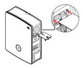
4 Check the replaced RCCB flap to ensure that it moves freely and then lock it with the key.
