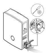
This completes the replacement of the charging socket flap. If necessary, repeat the procedure for the wallbox's second charging socket.
