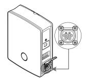
**2** Loosen the four screws with a Torx TR 20 screwdriver and pull the charging flap off the wallbox.
