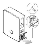
**3** Place the new charging flap over the frame of the Type 2 socket on the housing and screw it in place with the four screws supplied and the screwdriver.
